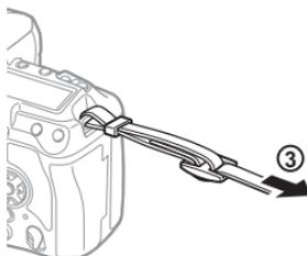
Lastly, pull the strap tight making sure that it is fastened securely (3).
