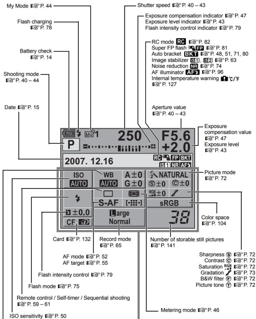
The functions within this area can be set on the super control panel.
