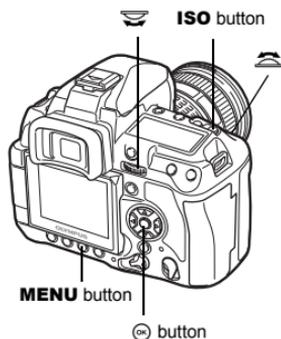
**[AUTO]** : The sensitivity is set automatically according to the shooting conditions. For **[ISO-AUTO SET]**, you can set the default (value normally used when the optimal exposure can be obtained) and upper limit (upper limit of ISO that automatically changes).
