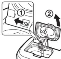
To attach the power battery holder to the camera, remove the camera's battery cover, as shown in the diagram to the left.
