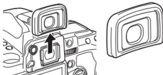
To remove the optional eyecup, remove it as shown on the left.
