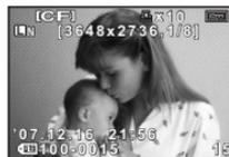
Displays the frame number, print reservation, protect, record mode, number of pixels, compression rate, date and time and file number
