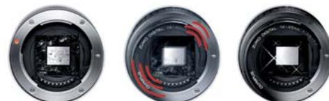
Dust particles have lodged on the dust filter in front of the sensor.
